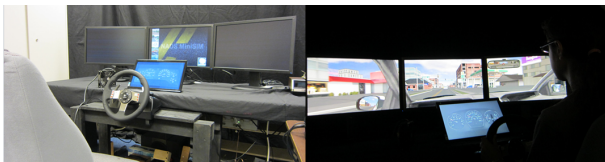
Fig. 3. Driving simulator at UMTRI where experiments were conducted. Twelve were under age 30 and 12 were older than 60.
