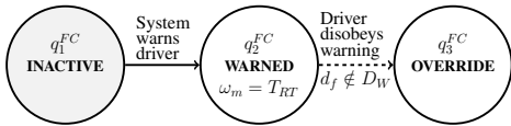
Fig. 2. Finite state machine corresponding to the modes of operation of the forward collision avoidance driver-assist system with events that trigger the mode transitions. The mode WARNED has non-zero minimum dwell time \omega_m .
